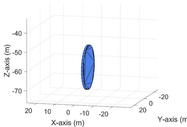
**Fig. 1** Example of 3-D panel for solving wave diffraction problem
